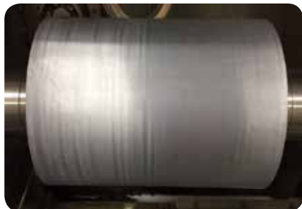
▲ Reserve Target Diameter for Rough Grinding Diameter + 1mm
