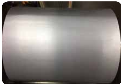
▲ TSKK is executed for 1mm removal quantity and sets the bed moving factor as 50mm/min. Exterior appearance, OK.
